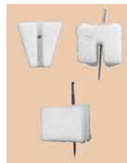
Figure 2: Brushite cement anchors used as bone-mimicking tissue supports during formation of the bone-to-bone ligament constructs.
